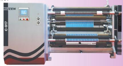
mum workable width is 600mm, which is also a unique feature that is difficult to find at most places. This machine has a very high operational accuracy with tolerances up to 0.25 mm. The Slitter Rewinder can be used with a wide variety of materials and is a completely automated machine with programmable logic control. MMI / HMI Color Touch Screen, Servo Controller, and Servo motors.
